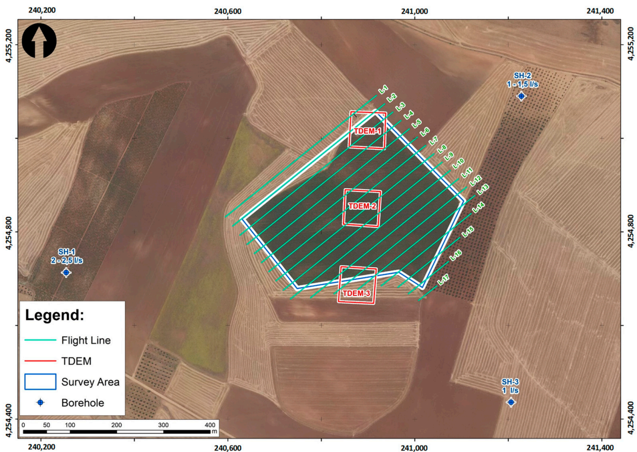
Figure 3. Flight plan made for magnetometry.
